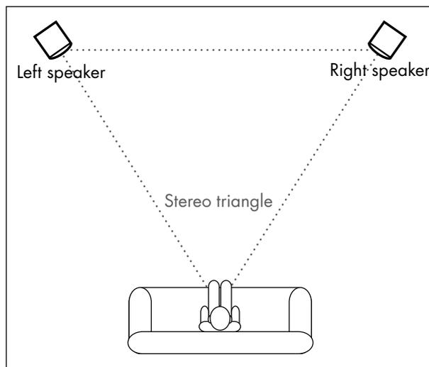
The speakers should be situated to the left and right of the listener and if possible, form an equilateral triangle with the listener – the so-called stereo triangle (distance from the listener = distance between the speakers). The speakers should project sound directly into the room or be arranged slightly towards the listener.
