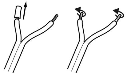
4. Turn the connector terminals counterclockwise until loose. Run the stripped single wire ends into the holes that are now visible. Turn the terminal clockwise until closed. The cable has now been clamped in place.
