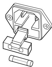
Push the old fuse out downwards. Insert a new fuse (2 A time-lag) and push the holder back. |
