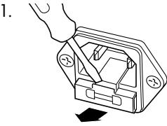
Remove the mains cable. Carefully pull out the fuse holder on the mains connection jack.       | 2.
